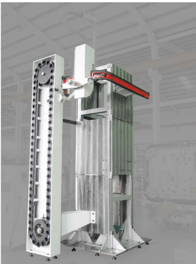
■ Vertical and horizontal tool changing system
