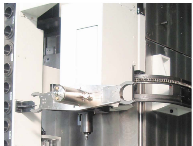
■ Vertical and horizontal tool changing system
